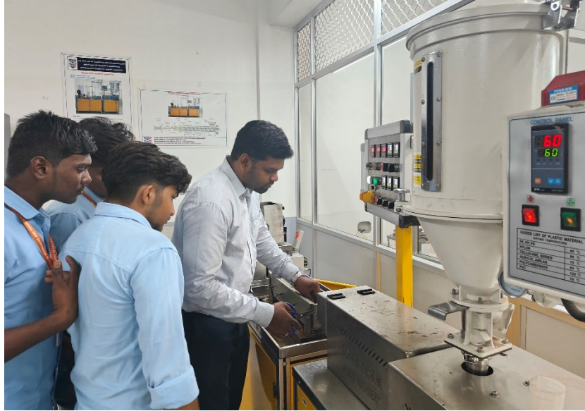
Mr Anto Dilip A, demonstrating the participants on the extrusion of 3D Printing filaments
